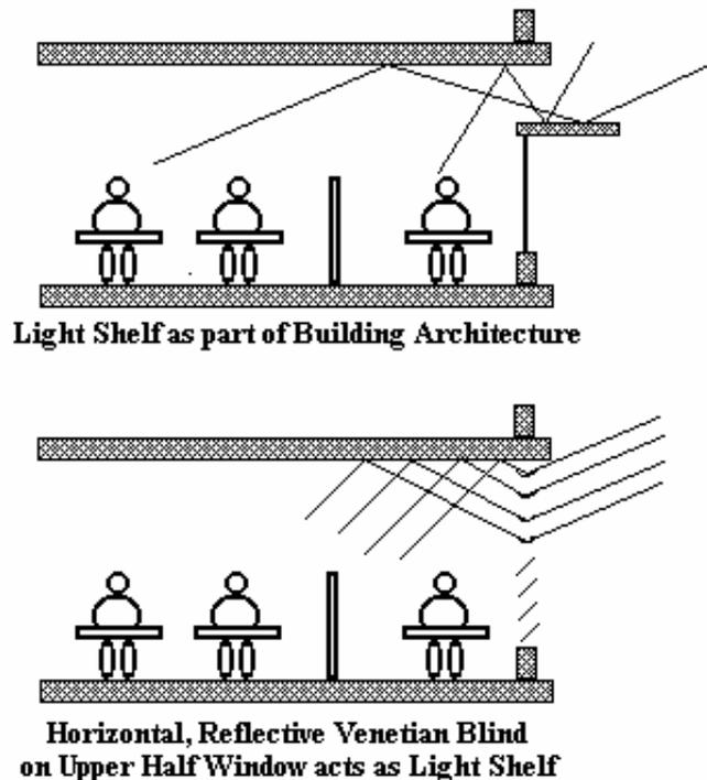
Figure 5-3: Concept of Light Shelf to provide Natural Lighting without Glare
