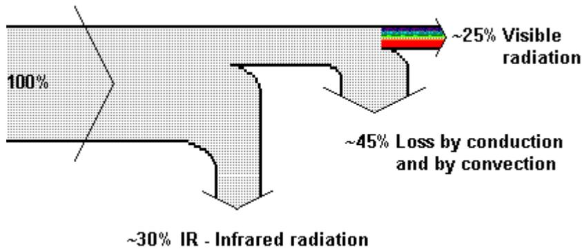
Figure 3-5: Energy flow diagram of fluorescent lamp
