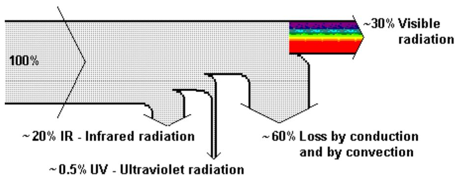
Figure 3-8: Energy Flow diagram of high pressure sodium lamp
