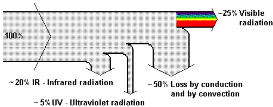
Figure 3-13: Energy flow diagram of metal halide lamp
