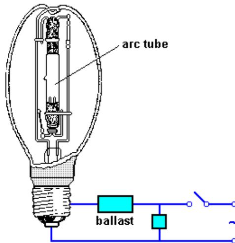
Figure 3-9: Mercury vapour lamp
