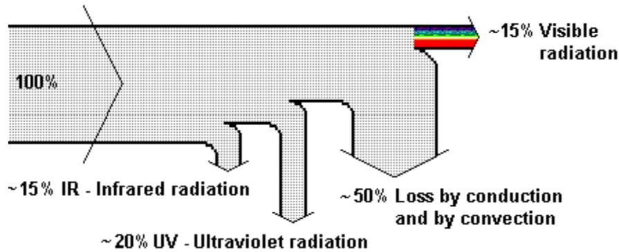
Figure 3-10: Energy flow diagram of mercury vapor lamp
