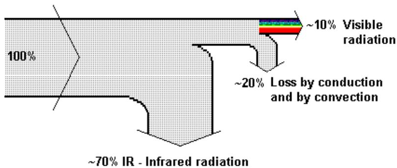
Figure 3-2: Energy flow diagram of incandescent lamp
