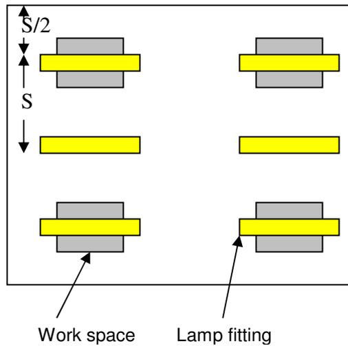
Figure 4-2: Luminaire spacing
