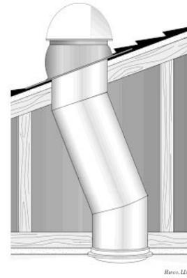
Figure 5-4: Light pipes
