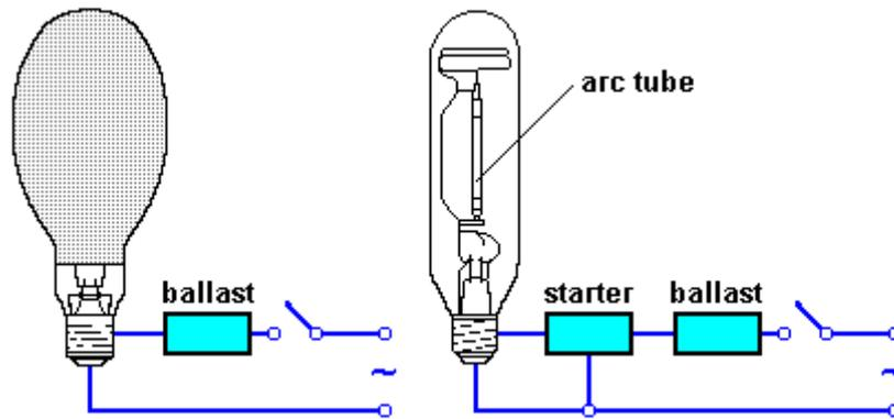
Figure 3-7: Sodium Vapor Lamp
