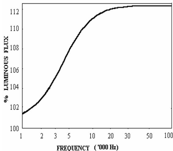
Figure 5-6: Increase in Light Output from Tube lights at Higher Operating Frequencies
