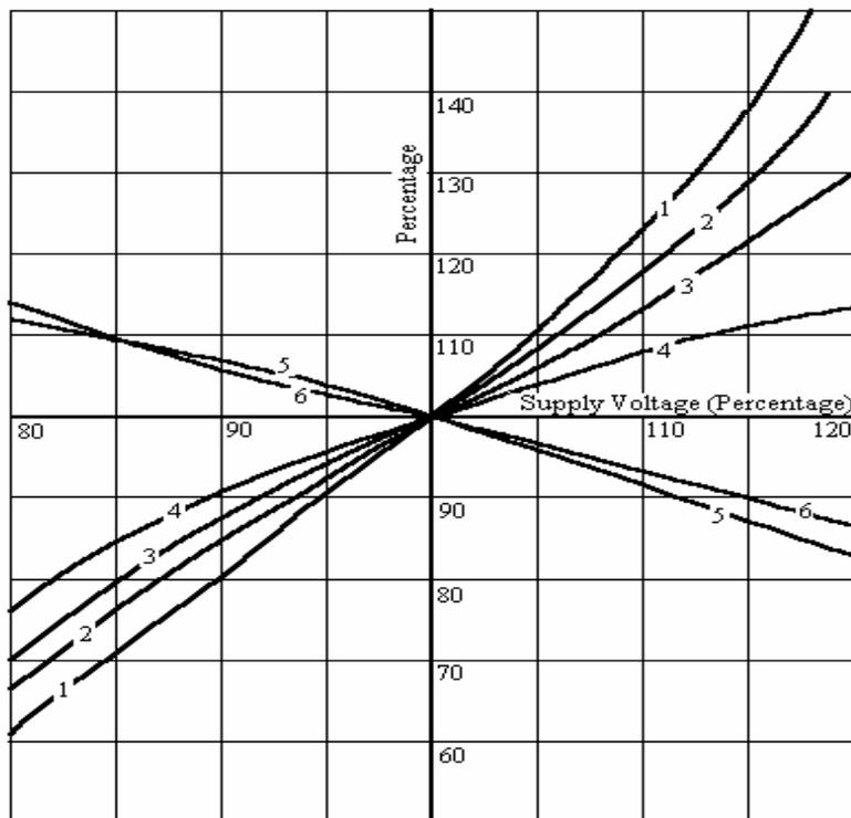
1. Lamp Current 2. Circuit Power 3. Lamp Power 4. Lamp Output
